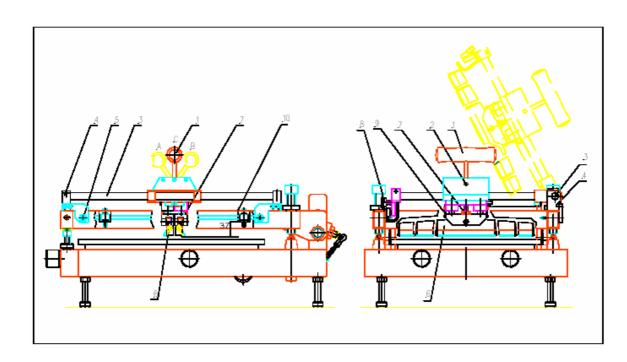
Printing with a squeegee guidance is offering the advantage to work user independent as squeegee pressure and angle are provided mechanically by the machine. Only the speed can be varied by the operator. The results are more repetitive and better printing results.
