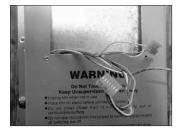
**5** Remove the switch box from the kiln by removing the screws holding the box to the kiln.
