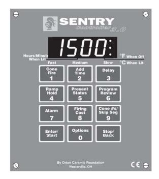
**Note:** In Program Review, Cone-Fire speed is displayed as the RA part of each segment. Cone-Fire Review shows the segments and ramp rates listed in the charts on pages 32 - 33.
