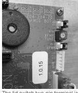
The lid switch two-pin terminal is on the back of the circuit board in the upper right corner.
