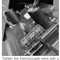
small slotted screwdriver. To avoid damaging the connection block, do not over-tighten the screws
