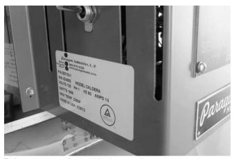
To figure the cost to fire your kiln, the controller needs to know how many kilowatts your kiln uses. Look at your kiln's electrical data plate for the watts and divide by 1,000. (Carry the decimal 3 places to the left. In the above photo, the wattage is 1680. Enter 1.68 in the KW option.
