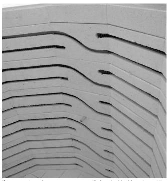
If you are not sure how many zones your kiln has, look inside and count the thermocouples. The kiln has a zone for each thermocouple. In this photo, the kiln is single-zone because it has only one thermocouple.
