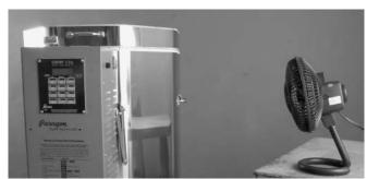
**Hot weather pointer**: Blow a gentle stream of air through the control panel of the kiln to reduce the temperature of the controller circuit board.
