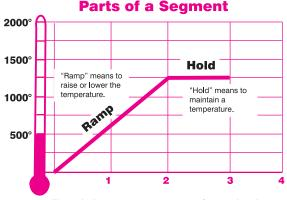
This segment will reach the target temperature of  $1250^\circ$  in 2 hours, then hold that temperature for 1 hour.
