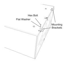
With assistance, carefully lift the air filtration system in place aligning drilled holes to mounting brackets. Bolt the air filtration system in place.
