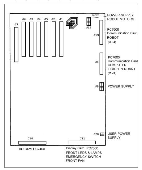
Figure 8-5: Main Board - Connectors
