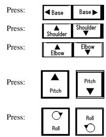
Before you press the keys shown below, make sure XYZ appears on the teach pendant display. Watch how the keys now affect the movement of the TCP.
