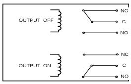
Figure 3-5: Relay Output States
