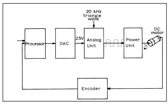
Figure A-5: Controller-A Control Loop
