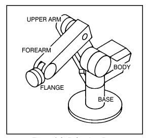
Figure 1-2: Robot Arm Parts
