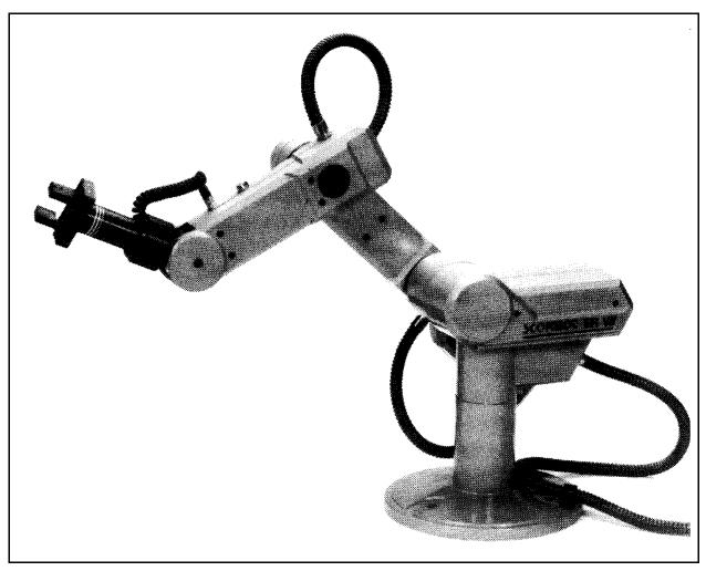
Figure 2-1: SCORBOT-ER VII Robot Arm
