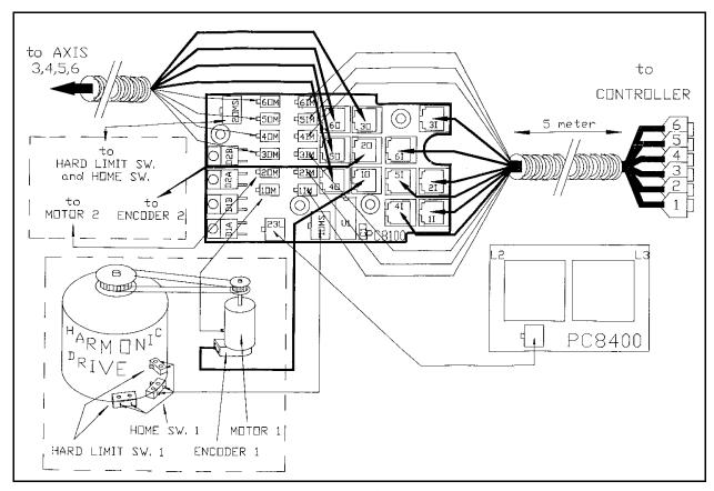
Figure 2-14: Robot Wiring
