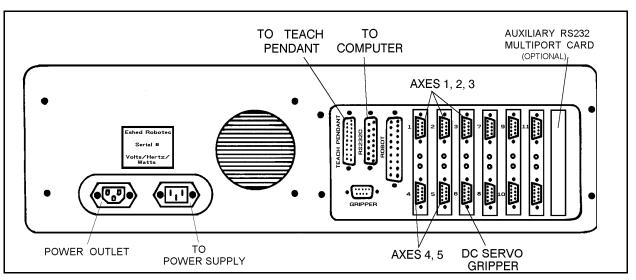
Figure 4-3: Controller Rear Panel
