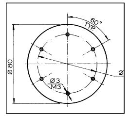
Figure 4-4: Gripper Mounting Flange
