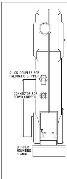
Figure 4-8: Gripper Connectors
