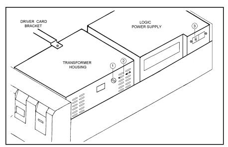
Figure 8-6: Controller Voltage Setting
