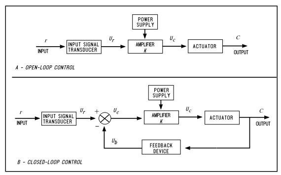
Figure A-1: Open-Loop and Closed-Loop Control
