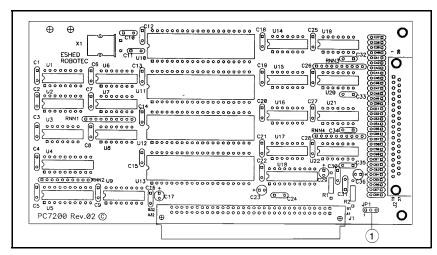
Figure 8-9: Auxiliary RS232 Communication Card
