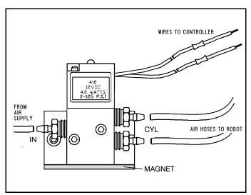
Figure 4-9: Pneumatic Solenoid Valve
