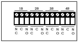
Figure 3-4: Relay Output Terminals
