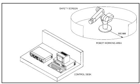
Figure 4-1: SCORBOT-ER VII Installation
