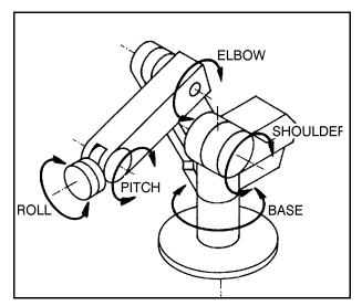
Figure 2-3: Robot Arm Joints
