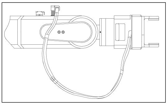
Figure 4-6: Connecting DC Servo Gripper - side view
