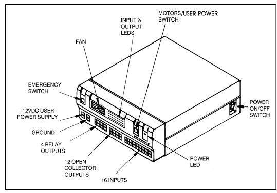
Figure 3-2: Controller Front Panel
