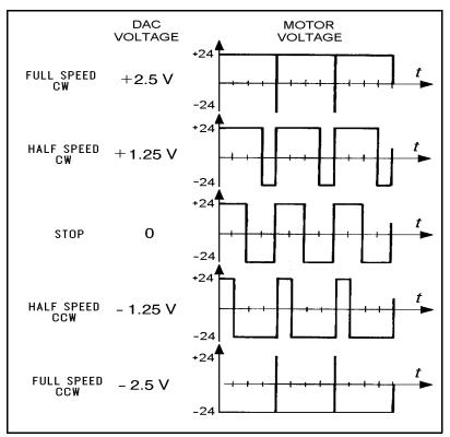
Figure A-6: Controller-A Control Signals
