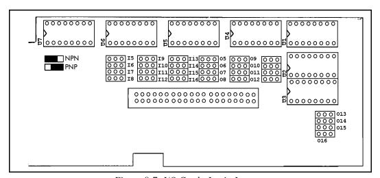
Figure 8-7: I/O Card - Logic Jumpers
