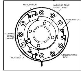
Figure 2-12: Microswitches on Axis
