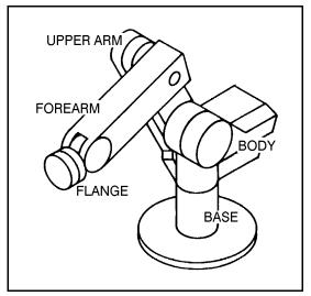
Figure 2-2: Robot Arm Links
