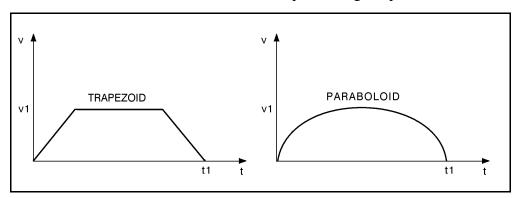
Figure A-7: Trajectory Control Profiles
