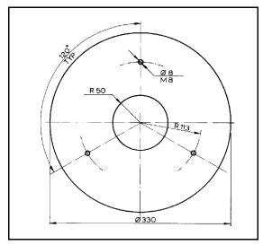
Figure 4-2: Robot Base Plate Layout
