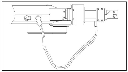
Figure 4-5: Connecting DC Servo Gripper - top view
