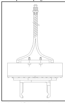
Figure 4-7: Pneumatic Gripper
