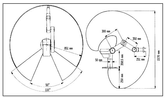
Figure 2-4: Operating Range With Gripper Attached
