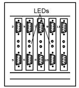
Figure 8-2: Driver Card LEDs
