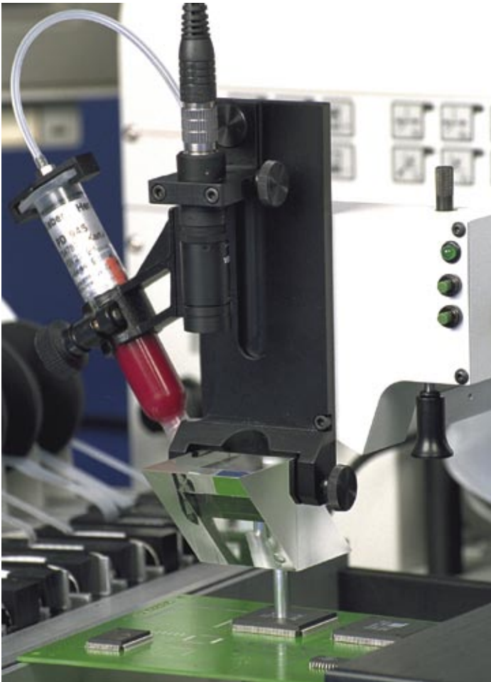
Fine pitch components are locked in a hovering position, exactly aligned and then automatically lowered to the PCB.
