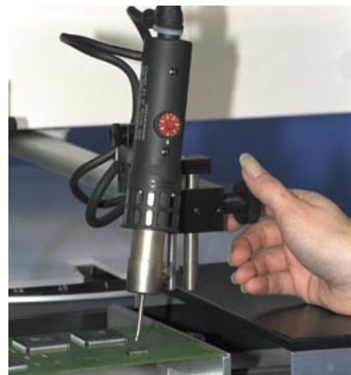
Optional hot air rework tool on second pantograph arm.
