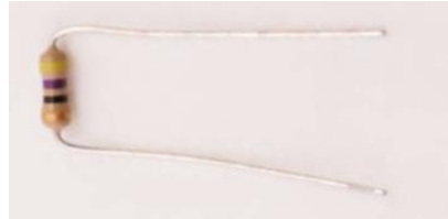
How to bend the leads of the resistor.
